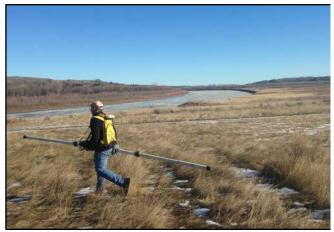
Using Electromagnetic Survey technology to locate buried arsenic bait along Missouri River.
