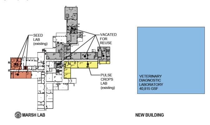
The final option is the construction of a new lab for the VDL. The new building would be a total of 40,815 gross square feet. This scenario increases the size of the VDL by 12,940 net square feet, this is slightly smaller than the original scope presented in the baseline, due to removing the food safety and DNA sequencing lab spaces since these are future functions desired by the agency. Also, the square footages of the BSL-2 enhanced necropsy and BSL-3 labs additions were slightly reduced.
