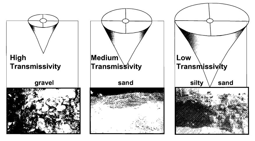
The more transmissive the aquifer, the smaller the cone of depression, all other things being equal. The size of the cone is a reflection of how much work it takes to move water to the well. It takes less work to push water through a coarse gravel than a silty sand.
