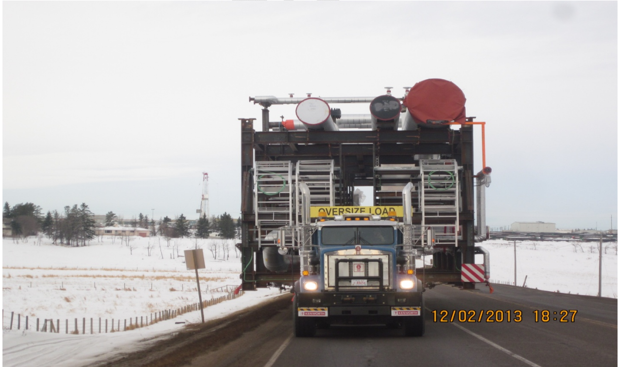
Front view of typical load size and transport equipment. Conventional trailer width allows for load to overhang edge of road while keeping transport vehicle and trailer on the pavement to facilitate traffic clearing on narrow roads.
