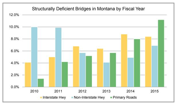
The above chart represents the percentage of structurally deficient bridges on Montana's highway systems, not including federally maintained bridges. A structurally deficient rating does not indicate that the bridge is dangerous for vehicular travel.
