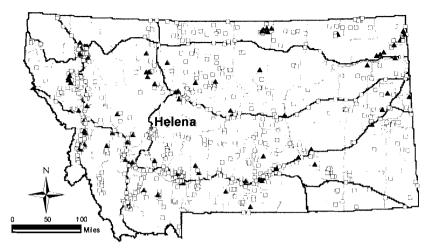
Quarterly water-level data from about 900 wells help people understand how the ground-water resource responds to climatic and other factors. Additionally, 100 water-level recorders (triangles) provide continuous or hourly data. Water-level data are available from the Ground-Water Information Center database.
