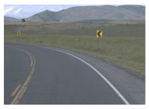
Enhanced delineation for horizontal curves is often considered with pavement markings, post-mounted delineation, larger signs and signs with enhanced retro reflectivity and dynamic advance curve warning signs and sequential curve signs. Chevron signs have been proven to reduce nighttime crashes by up to 25 percent.
