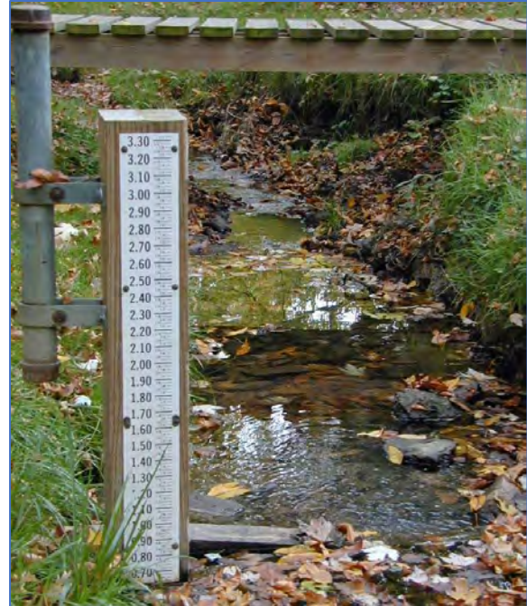
Figure 16: Staff gage coupled with a crest stage gage (left hand side of photo). Source: USGS
