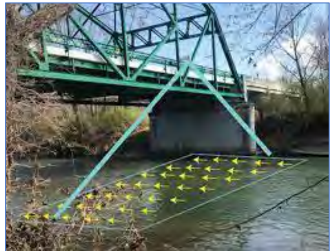
Figure 17: Large -Scale Particle-Image Velocimetry (LSPIV) uses video to capture particles on the surface of the water passing beneath the instrument. Source: USGS
