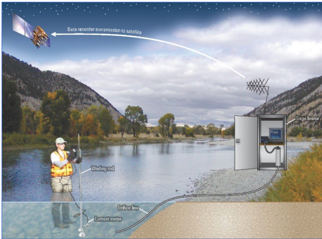
Figure 2: Diagram of typical stream gage installation with equipment used to measure stage and take physical discharge measurements to maintain the validity of the rating curve. Source: USGS
