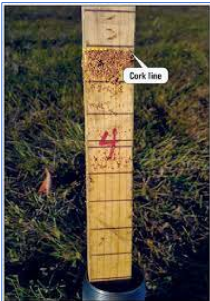
Figure 15: The cork line marks the maximum water level in a crest stage gage. Source: USGS
