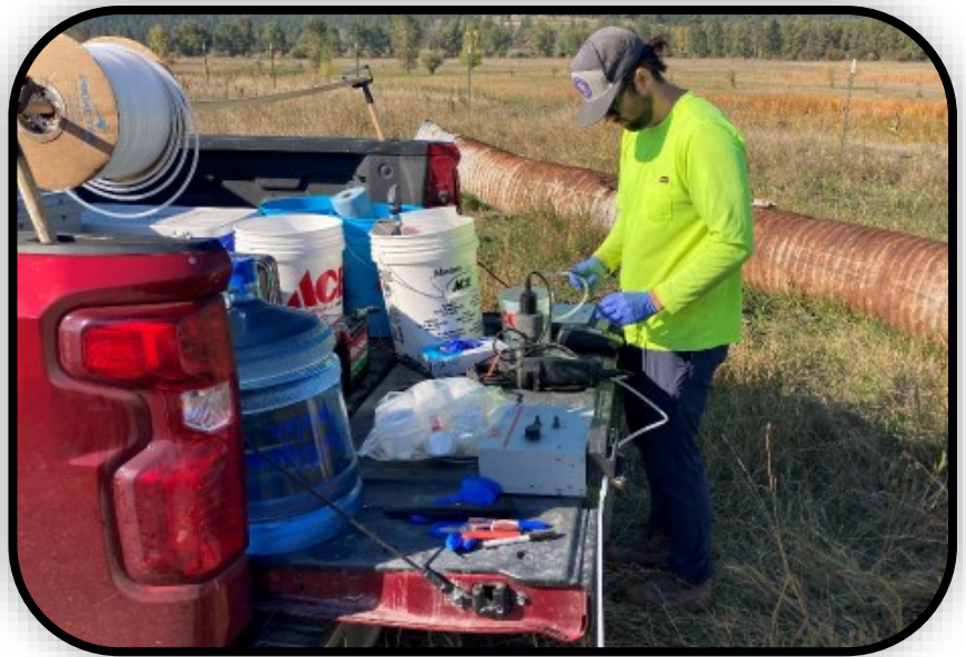
Typical groundwater sampling set up.
