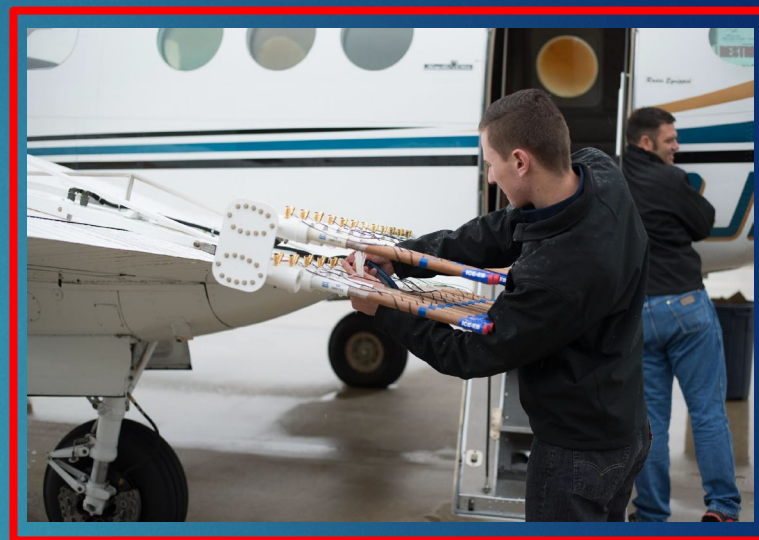
Wing mounted "Burn-in-Place" (BIP) flares
